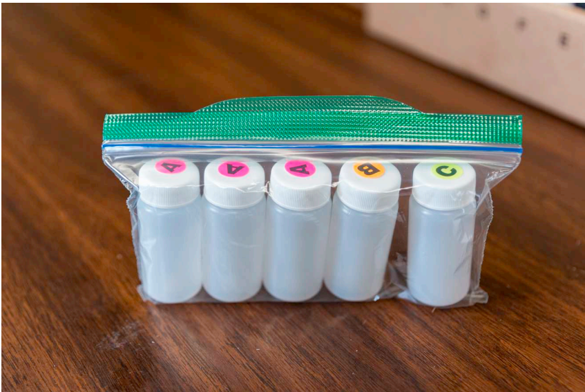
FIGURE 4 Plastic vials for lead testing to be distributed to community citizen scientists.
