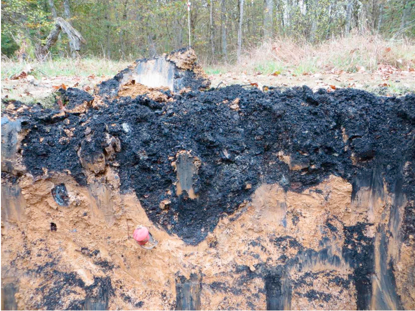
FIGURE 1 Place à Gaz. Cross-section of a trench shows the residues of Blackened Open-burning (OB) chemical shells overlying compact clay. (D Hubé, October 2014).
