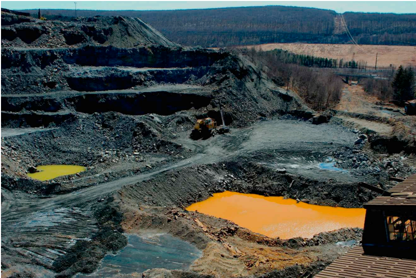
FIGURE 15.3 Acid mine drainage near Mahanoy City, Pennsylvania. This orange water has high levels of iron hydroxide, a common feature found in waters impacted by mine water runoff. While this pool is found in a strip mine, the impact of acid mine drainage can be found throughout the anthracite region (Courtesy Gabby Zawacki, 2016).
