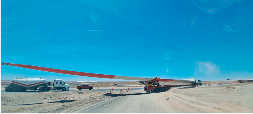
FIGURE 7.3 Transporting a windmill blade of a wind turbine generator, by the authors.
